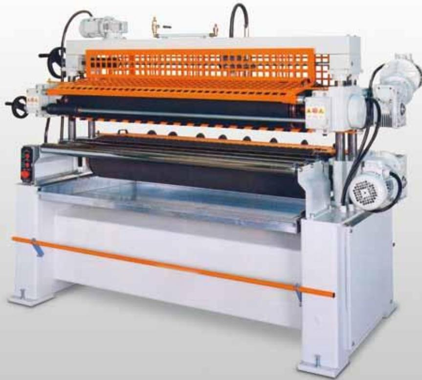
**DOSING ROLLERS** made of ebonite 180 mm diameter; they are revolving at lower speed than spreading rollers, so glue is distributed only to the spreading rollers when they'll be in contact by means of a free wheel device. The peripheral speed conforms eliminating the overheating and rubber wearing.
